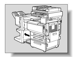
2 Pull out the hole-punch waste container.
